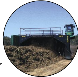
ALLU AS Windrow turner - mixing soil and binding agent in large volumes
