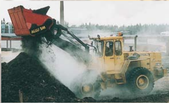
2. Aeration of sludge compost speeds up the composting process.
