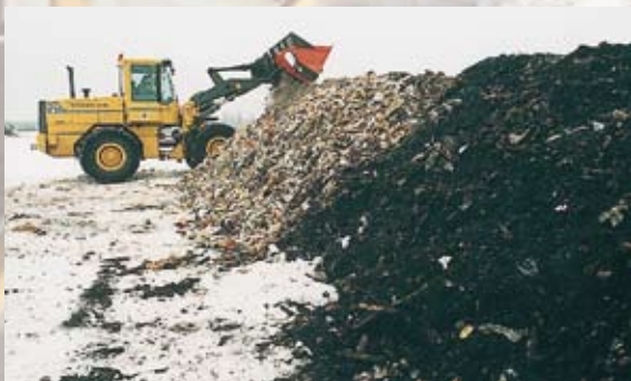
3. Biowaste and the bulking agent can be crushed and mixed in one step.
