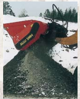
13. Crushing of light-weight concrete.
