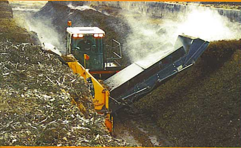
>> Rotation and oxygenation, in particular of compost stacks, contaminated soil and in mechanical-biological treatment systems
