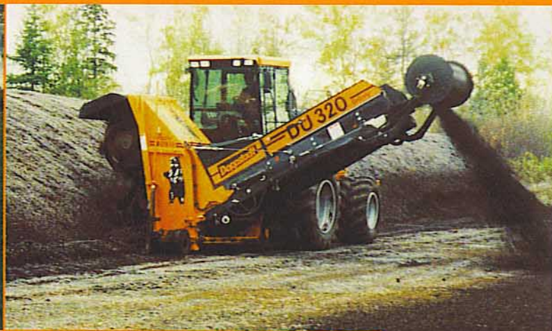
>> Rotation and oxygenation, in particular of compost stacks, contaminated soil and in mechanical-biological treatment systems
